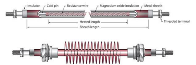
Finned tubular elements are made of Incoloy 800 (Nickel-Alloy) tube with a diameter of 3/8" (9.5mm). Neptronic uses precision wound 80-20 nickel-chrome wire to deliver an
