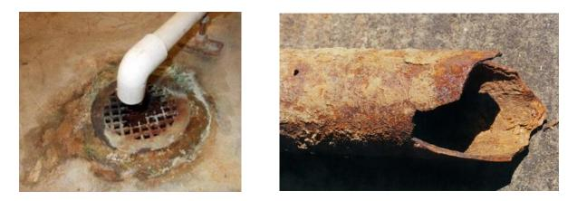
The acidic level of the condensate is measured in pH on a scale from 0 to 14. Most condensate will have a pH between 2.9 and 4 (according to the actual chemical makeup of the fuel that is being burned) with 7 being neutral. This scale is not linear; each step below 7 is 10 times more acidic than the next higher number. Treated condensate should be as close to neutral as possible with 5 being the minimum.
